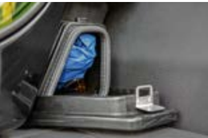
• Storage compartment for gloves and protective clothing • Keeps PPE out of the Cat 4-certified cab
